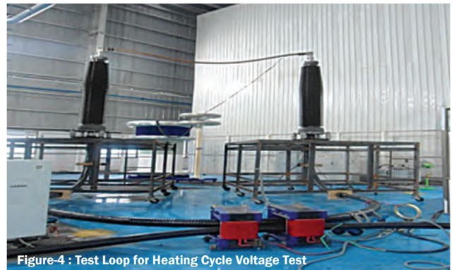
Figure-4 : Test Loop for Heating Cycle Voltage Test
