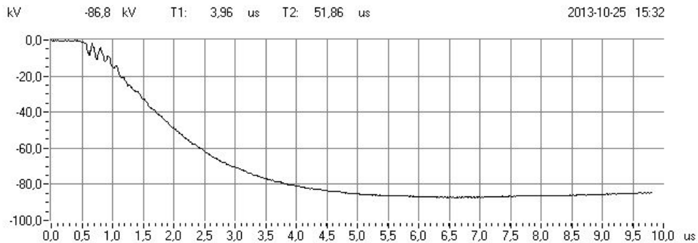
Fig. 5: Waveshape 72122084, KEC, -50% of test voltage
